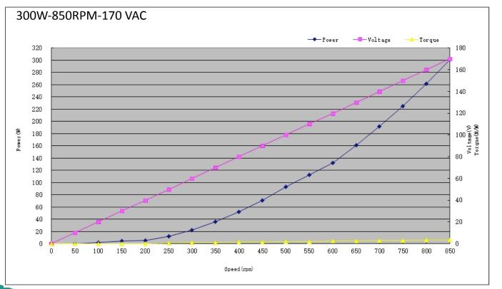
Power curve by Aeroleaf (without petal) Voltage / Power / Rotation speed
